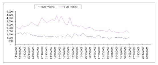
Since 14/09/2008 transducer Nulls ("No Answers") have been reduced by 550, while transducers reading less than 3 lbs of pressure have been reduced significantly from a high of 4,393 on 23/01/2009 to 1,804 on 13/09/2009. These results coincide with Monitronix RMU and DFP installations.
